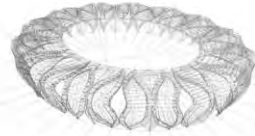
6. Secondary structural elements for lateral bracing and roof systems are linked to the primary truss system.
