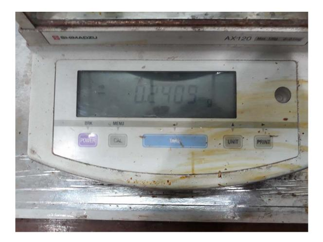
Figure 3: Control Fields and Display of AX120 Electronic Balance
