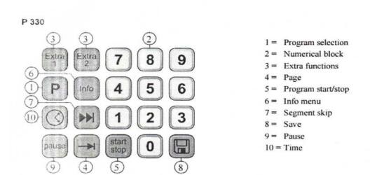
Figure 7: P330 Keyboard Block
