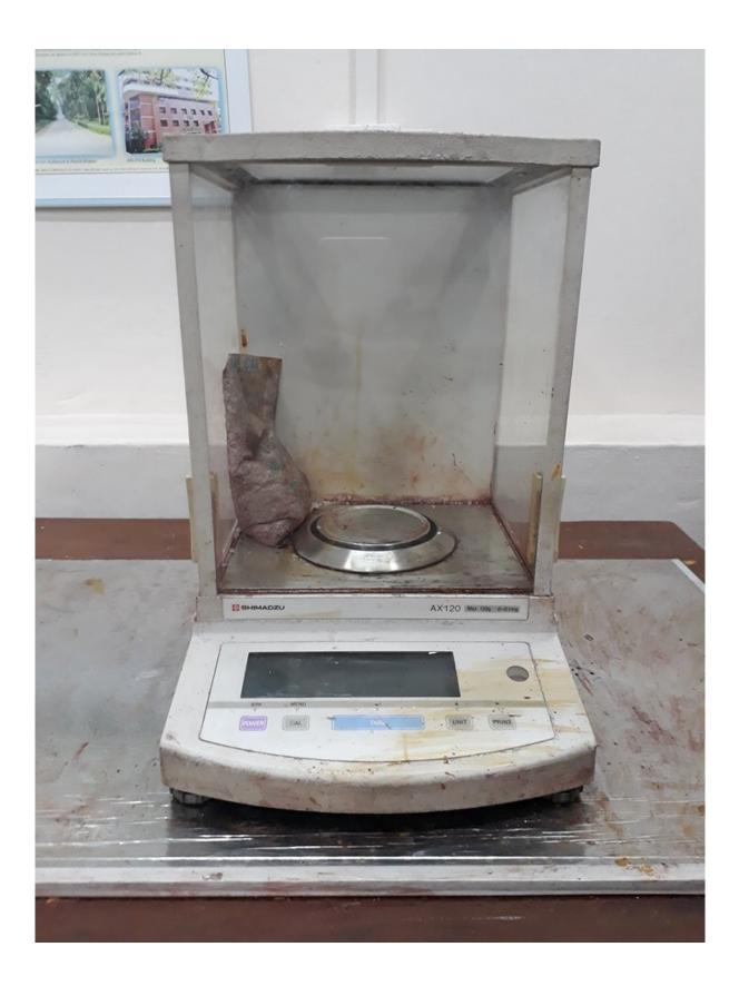
Figure 2: AX120 Electronic Balance
