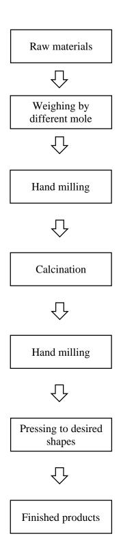
Figure 1: Flowchart of the stages in preparation of spinel ferrite
