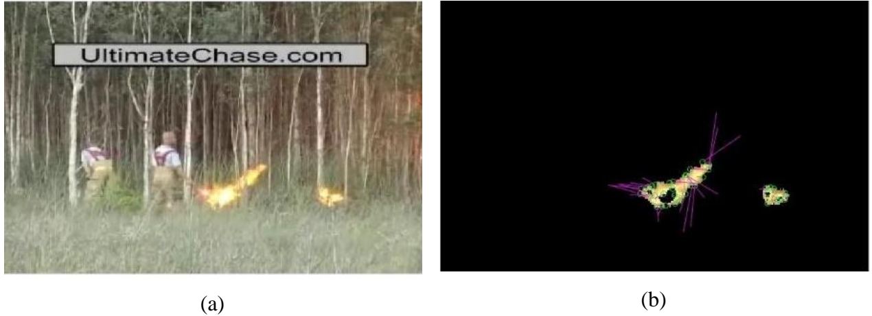
Figure 17. (a) Shows the original frame from a video with fire in outdoor condition. (b) Shows the velocity vectors calculated of corners detected in the flame region in (a).
