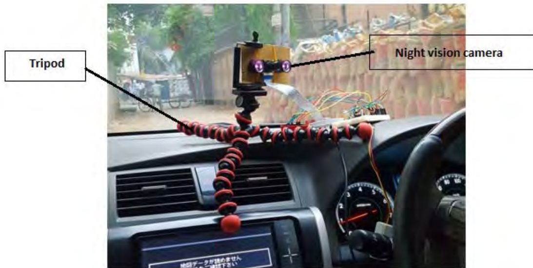
Figure 25: Placement of the night vision camera
