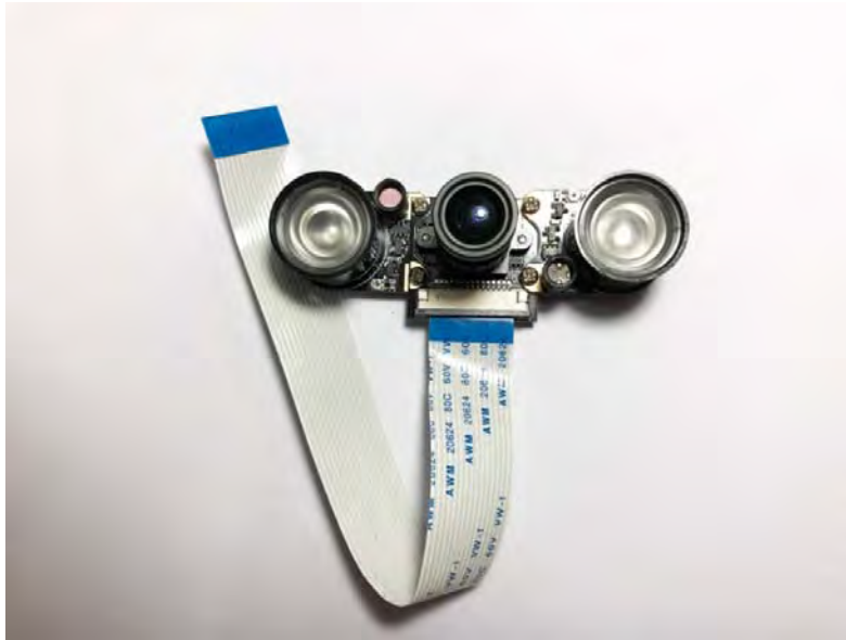
Fig 12: Raspberry Pi night vision camera
