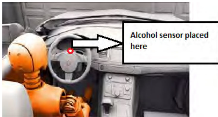
Figure 32: Placement of alcohol sensor on steering wheel
