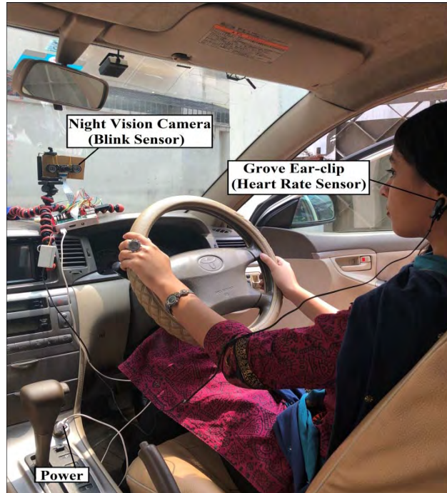
Figure 26: Implementation of the system in the car
