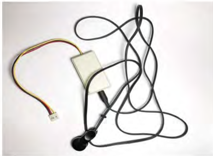
Figure 04: Grove ear clip heart rate sensor
