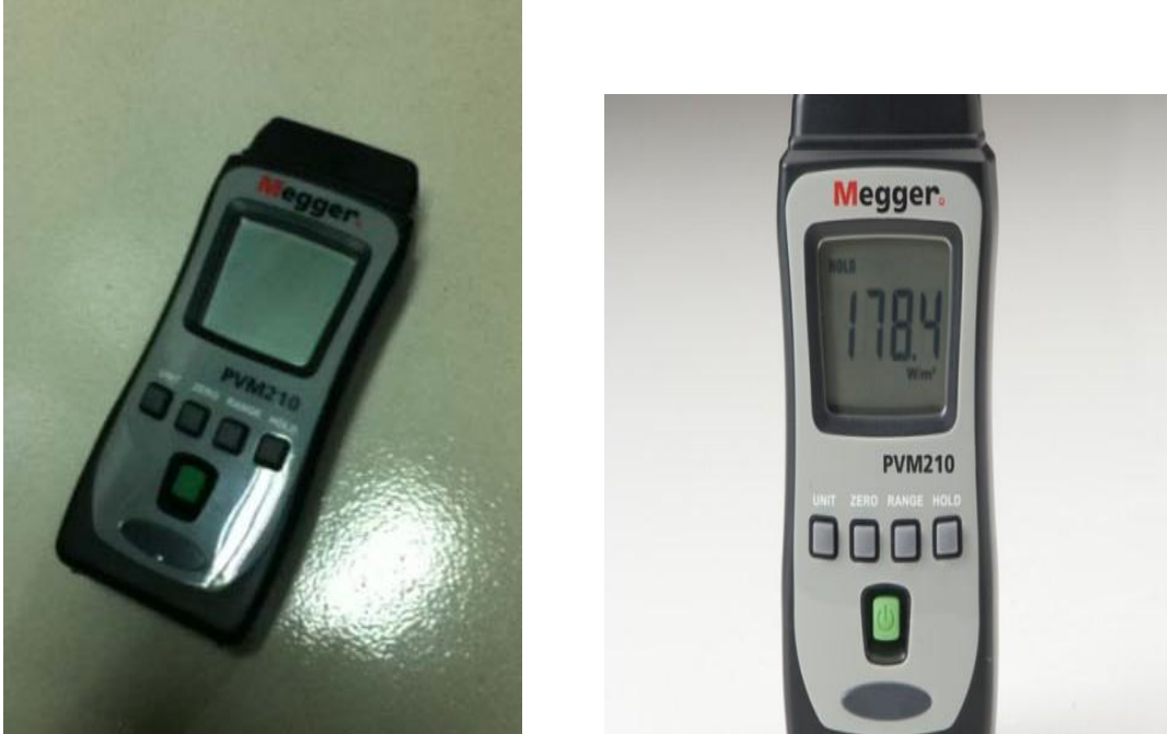
Figure 6.2.1: Megger PVM210 Irradiance meter
