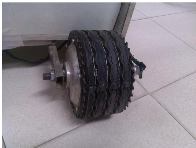
Fig. 13 HUB motor with CNG rubber tire attached
