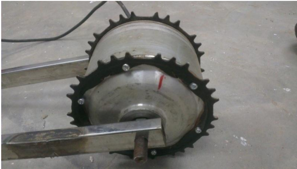
Fig. 4 HUB motor with sprocket
