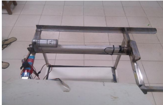
Fig. 14 Single Linear Actuator with supporting stands
