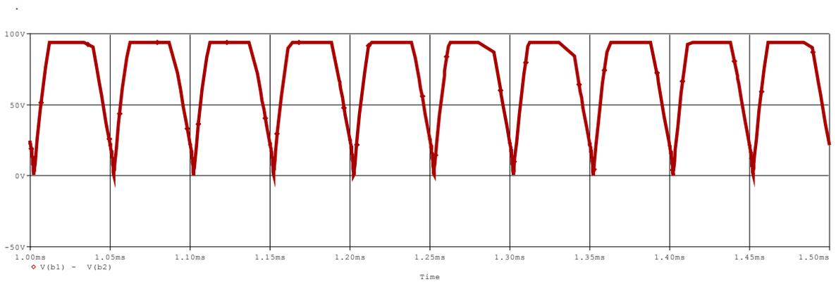
Figure 3.4(c): Output Wave Shape of Series Resonant Dc-Dc Converter
