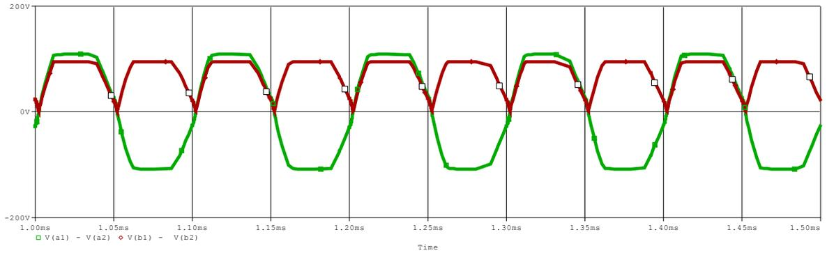
Figure 3.4(d): Combined Wave Shape of Inductor-Capacitor & Output.
