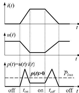
Figure 1.2(b): Power losses in real switches
