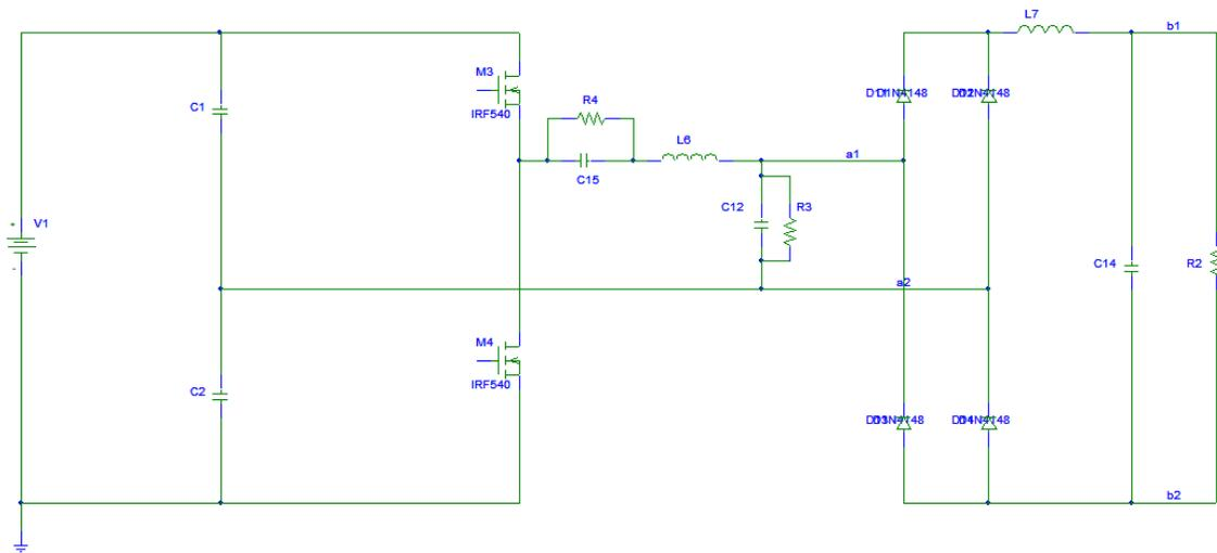
Figure 3.7: Series-Parallel Resonant Dc-Dc Converter.
