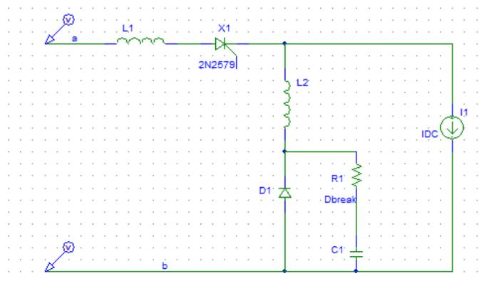
Figure 1.3(b): Diode Snubber Circuit
