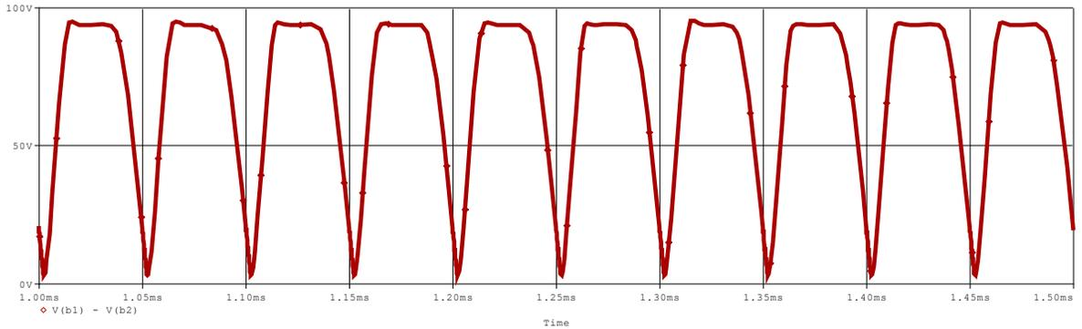
Figure 3.8(c): Output wave shape of Series-Parallel Resonant Dc-Dc Converter.
