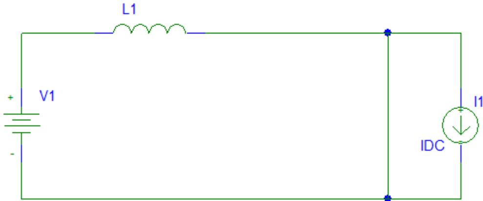
Figure 2.2(d): Switch Closed and D2 On
