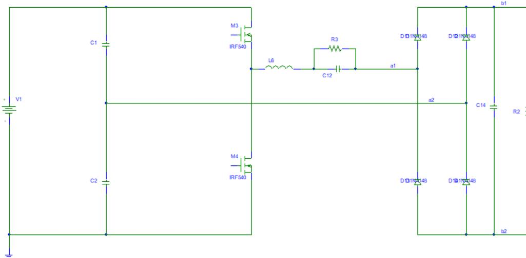
Figure 3.3: Series Resonant Dc-Dc Converter.
