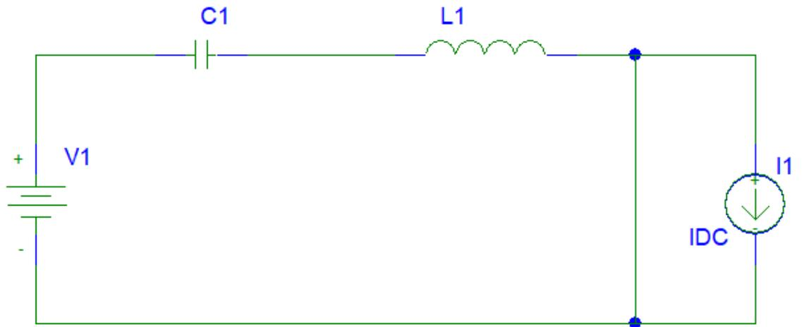
Figure 2.2(c): Switch Open and D2 on
