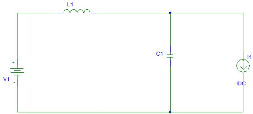
Figure 2.1(c): Switch Closed and Diode On ( $0 < t < t_1$ )
