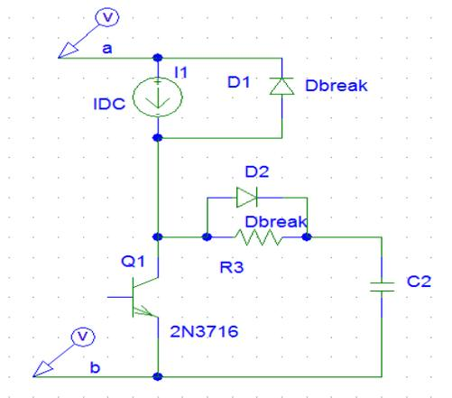
Figure 1.4(a): Turn On Principle Using BJT
