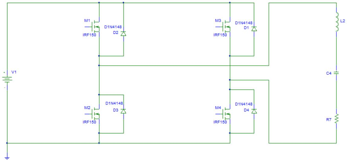
Figure 3.1: Series Resonant Dc-Ac converter.
