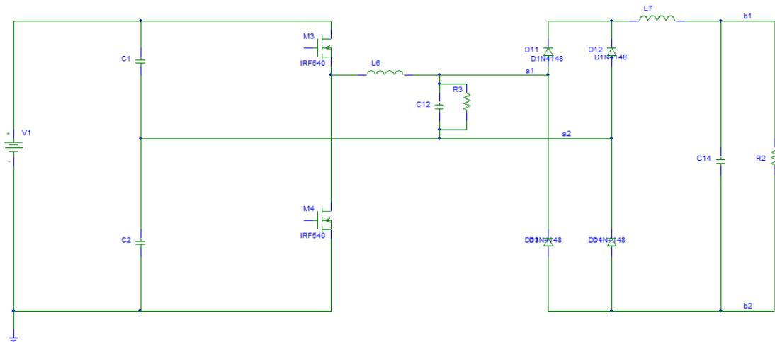
Figure 3.5: Parallel Resonant Dc-Dc Converter.
