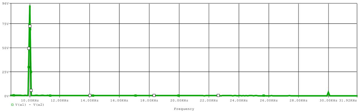
Figure 3.6(b): F.F.T of Wave Shape Across Inductor And Capacitor.
