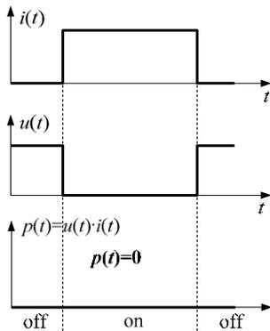
Figure 1.2(a): Power losses in ideal switches
