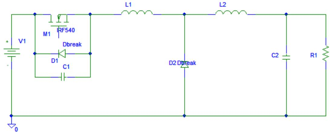
Figure 2.2(a): A Resonant Converter with Zero-Voltage Switching
