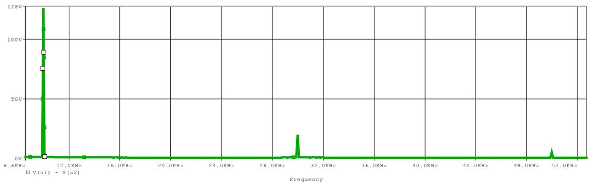
Figure 3.4(b): F.F.T of Wave Shape Across Inductor And Capacitor.
