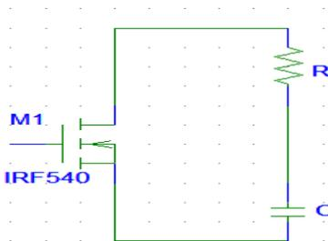
Figure 1.4(b): Turn Off Principle Using MOSFET
