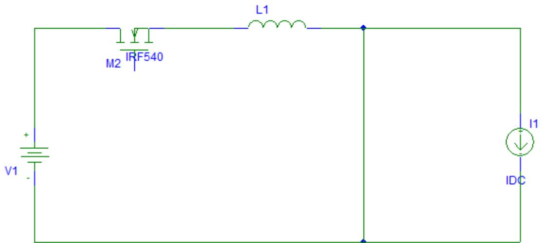
Figure 2.1(b): Switch Closed and Diode On ( $0 < t < t_1$ )
