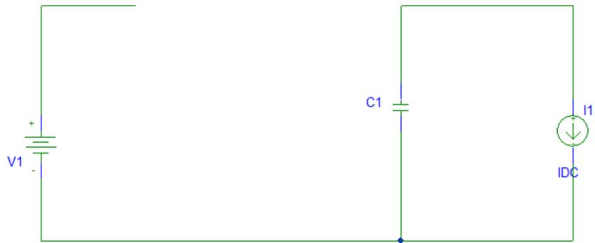
Figure 2.1(d): Switch Open and Diode Off
