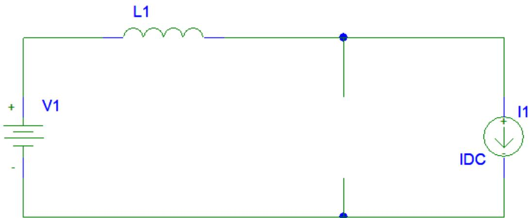
Figure 2.2(e): Switch Closed and D3 Off( $t_3 < t < T$ )
