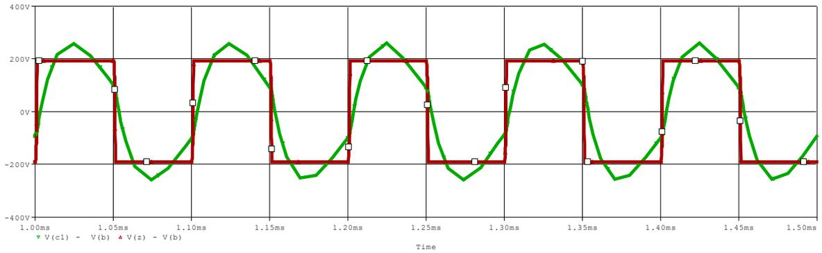
Figure 3.2(d): Series Resonant Dc-Ac Converter (input & output)
