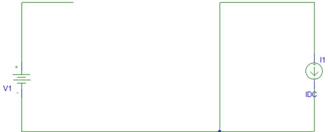
Figure 2.1(e): Switch Open and Diode On ( $t_3 < t < T$ )
