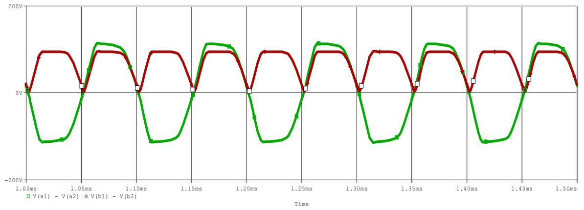
Figure 3.8(d): Combined Wave Shape of Inductor-capacitor & output.
