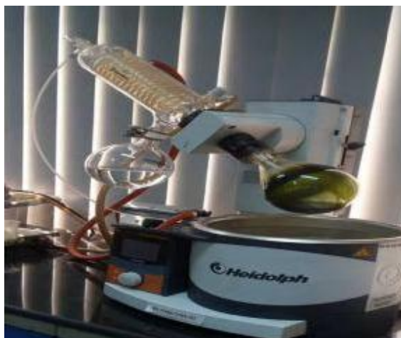
Figure 2.6: Concentrate the filtrate of the Aporosa wallichii plant using an evaporator rotator
