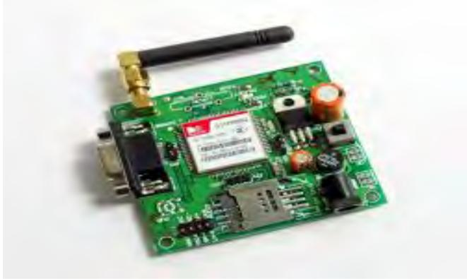
Figure 3.5: GSM Module
