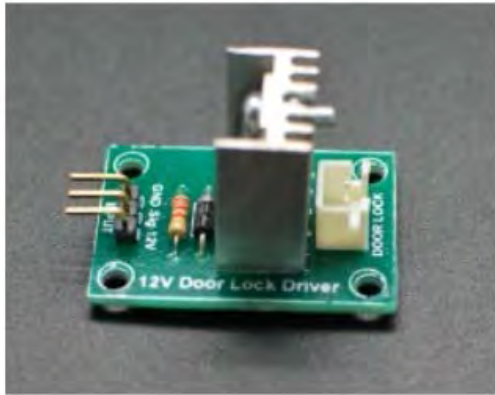
Figure 3.3.19 12V door lock driver
