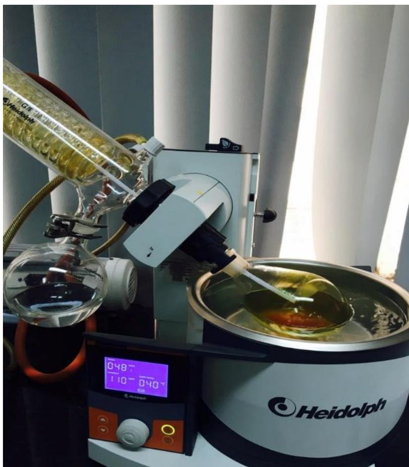
**Figure 3.1** Rotary vacuum evaporator
