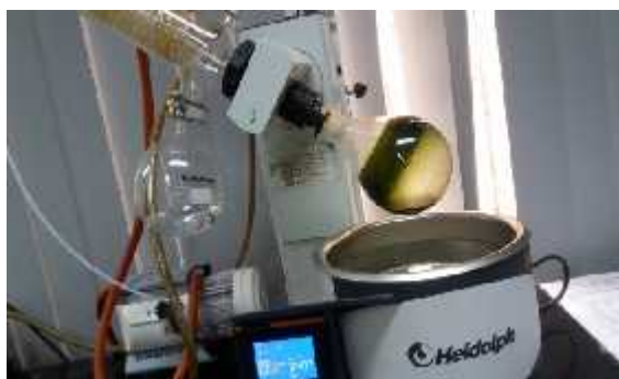
Figure2.2: Evaporation in the rotary evaporator
