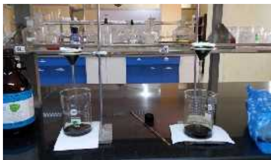
Figure2.1: Filtration of the methanolic extract
