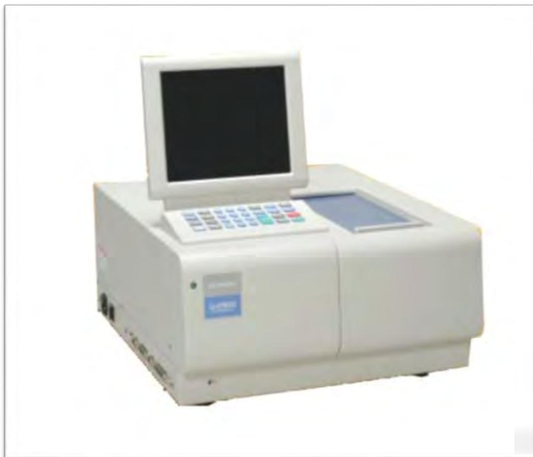
**Figure 2.2:** UV Spectrophotometer
