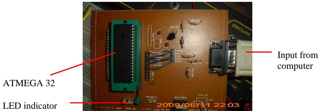
**Fig 11:** The downloader Circuit
