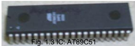
Fig. 1.3 IC: AT89C51
