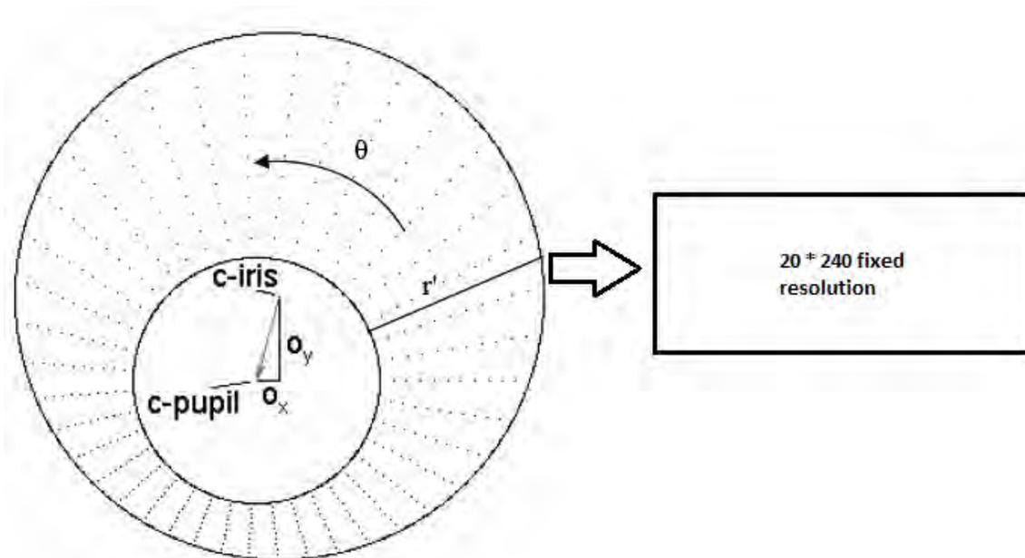
Figure 7: The doughnut form iris region is transformed into a rectangular normalized 2D array [1].
