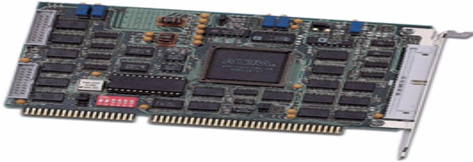
*FIGURE 3.4: AX5411H DAQ Board*
