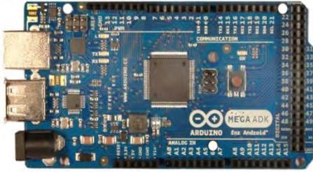
**Fig 19: Microcontroller Arduino ADK**
