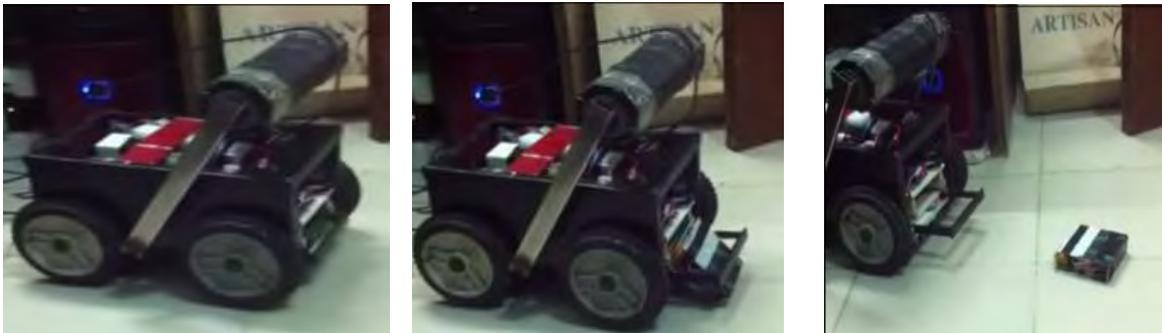
**Fig 10: Beacon Deploy Mechanism**
