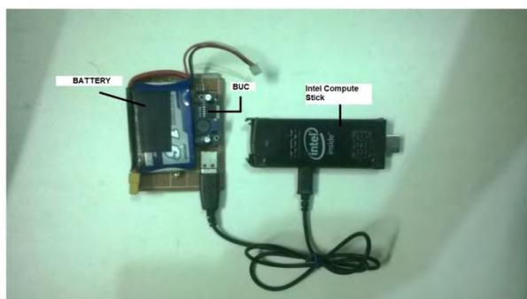
**Fig18: Customized power bank powering Compute Stick**
