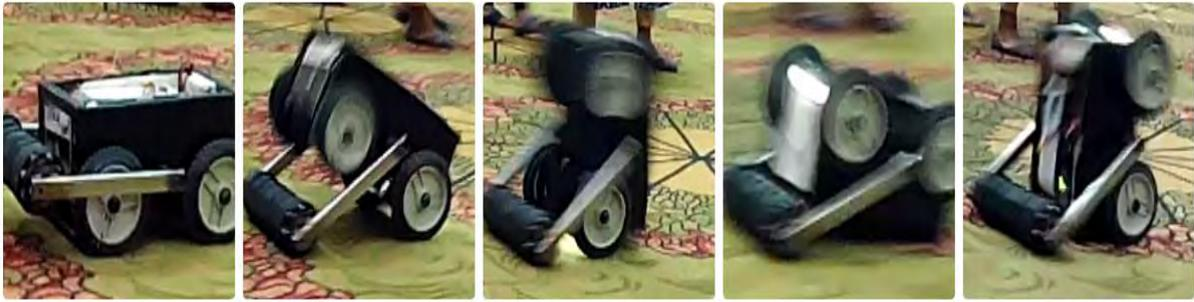
**Fig 11: Rescue Robot in motion, taking flips using wedge**
