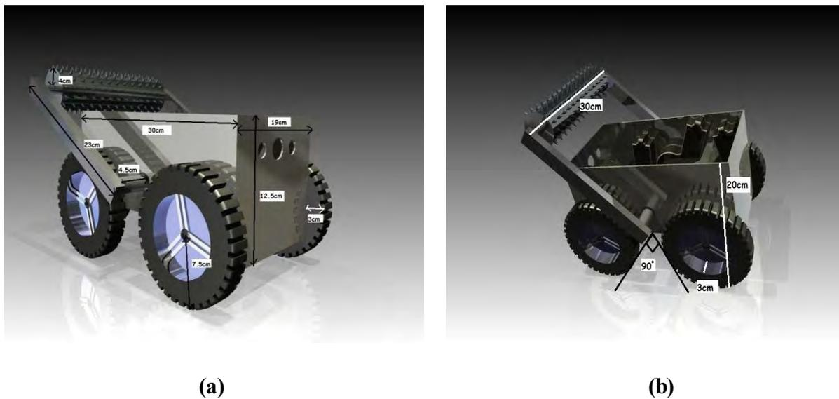
**Fig 6: CAD diagram with measurements**
