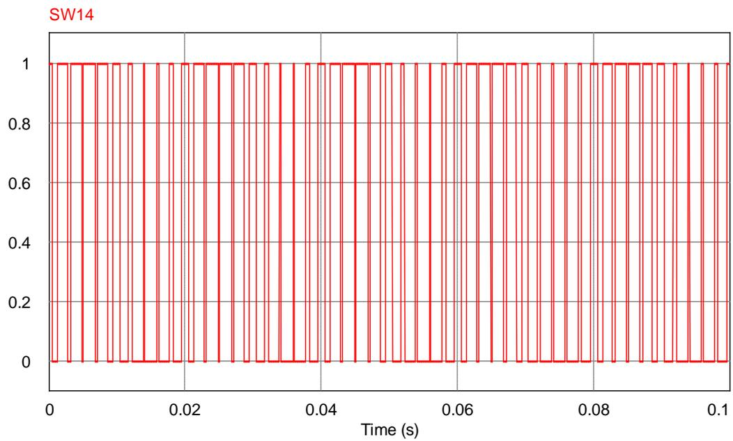
Figure 3.6.2: Switching signals for Switch 1 and 4
