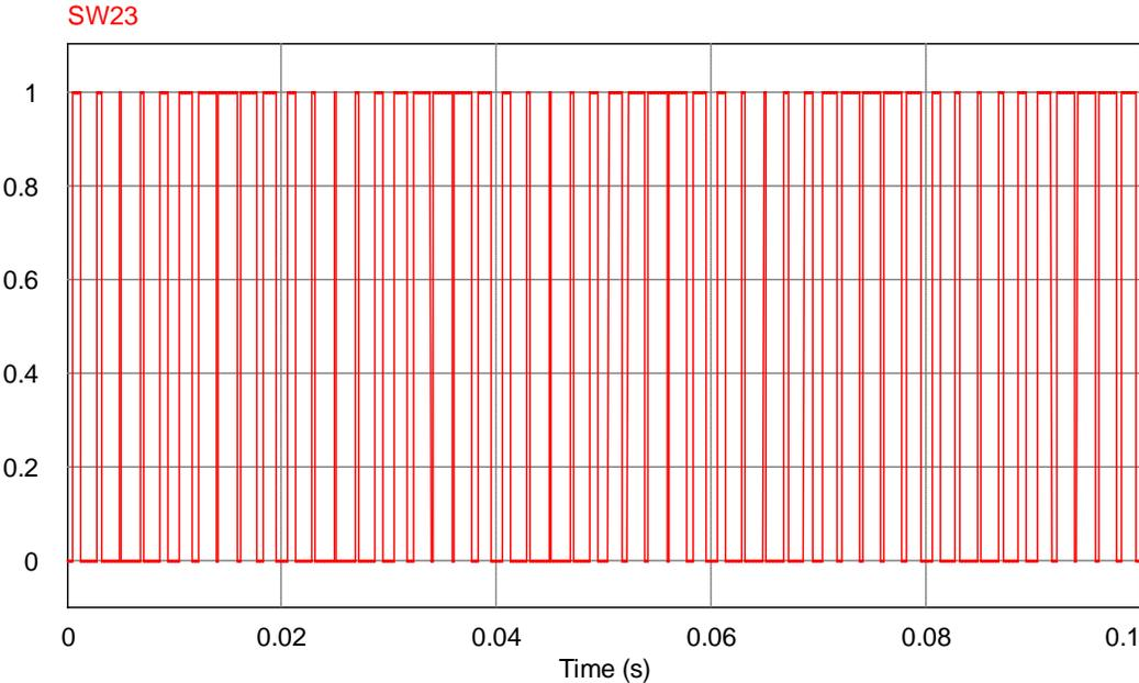
Figure 3.6.3: Switching signals for Switch 2 and 3
