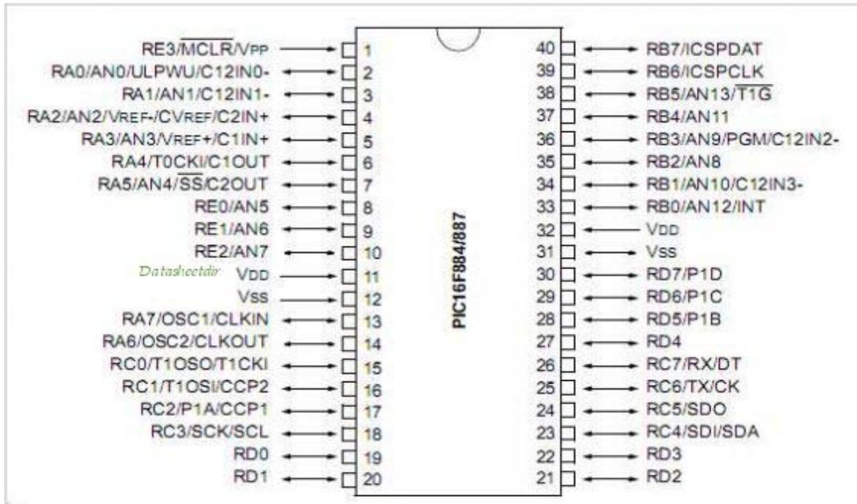
Fig 2.4: 40 Pin PIC16F887 pin Assessment
