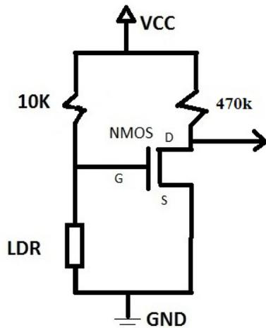
Fig 3.5: The Diagram shows LDR Construction for this Project
