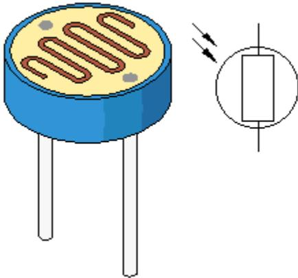
Fig 2.2: Light dependent Resistor
