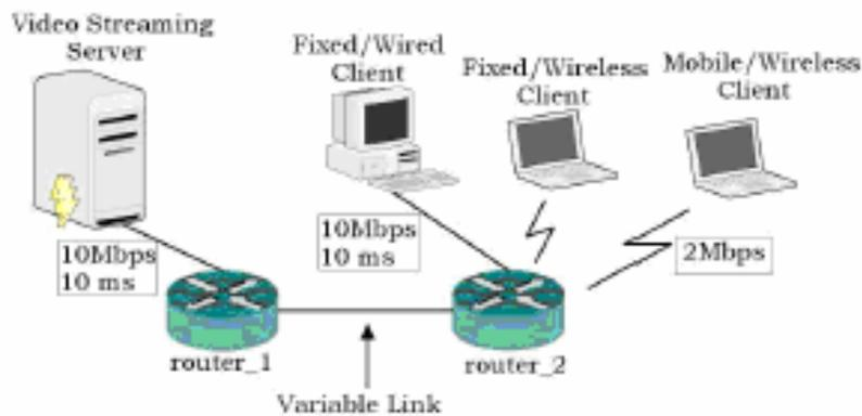
**Fig 2: Video Stream Evaluation Setup.**
