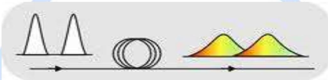
Fig 2.3: A pulse broadens due to chromatic dispersion
