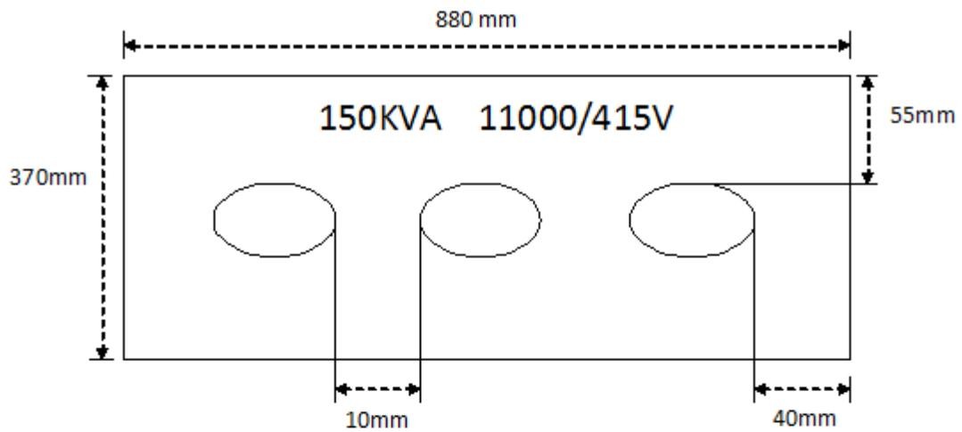
Figure: Side view of a transformer
