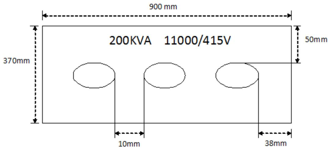
Figure: Side view of a transformer
