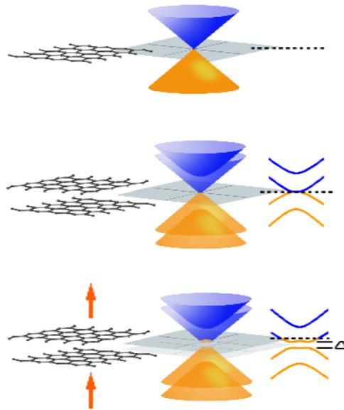
**Fig11: One of the most unusual features of single-layer graphene (top) is that its conical conduction and valence bands meet at a point – it has no bandgap. Symmetrical bilayer graphene (middle) also lacks a bandgap. Electrical fields (arrows) introduce asymmetry into the bilayer structure (bottom), yielding a bandgap ( $\Delta$ ) that can be selectively tuned<sup>21</sup>.**
