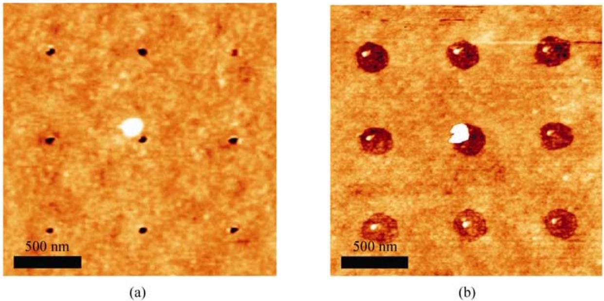
**Fig-2: (a) The result fo AFM indentation of a 3 × 3 matrix of holes in graphene. (b) AFM micrograph of the hexagonal holes grown from the defects induced by indentation. Protrusions inside the hexagons are remnants of the AFM indentation process <sup>13</sup>**
