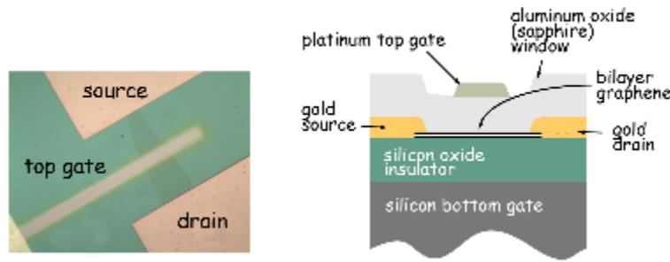
**Fig12: From left, a microscope image looking down through the bilayer-graphene field-effect transistor. The second one displays the elements of the device <sup>21</sup>.**
