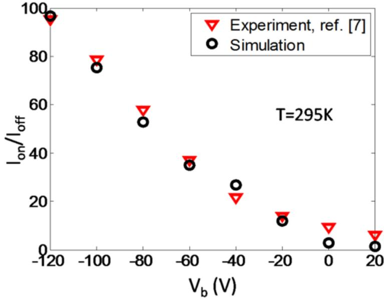
**Fig-10:** On/off current ratio as a function of the back gate bias voltage ( $V_b$ ). Experimented values almost match the simulation values. There's only a slight mismatch between the experimented and simulated values<sup>15</sup>.
