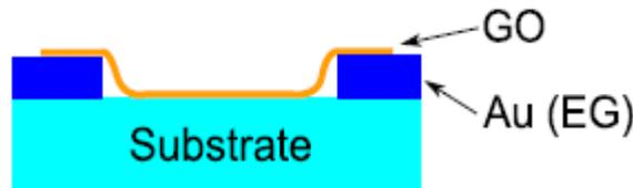
**Fig3:** A side view of the layout of GO devices
