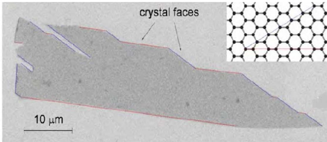
**Fig8. Scanning-electron micrograph of a relatively large graphene crystal, which shows that most of the crystal's faces are zigzag and armchair edges as indicated by blue and red lines<sup>2</sup>**
