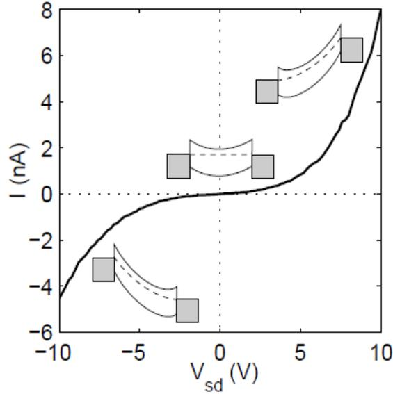
**Fig5: I-V characteristics of an 800nm device. The asymmetry reflects dissimilarities of the two junctions<sup>11</sup>**
