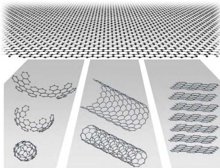
**Fig1:** All graphicitic forms. 2D Graphene that can either be wrapped up into 0D buckyballs or can be rolled into nanotubes. Also can be stacked to form 3D graphite<sup>2</sup>.
