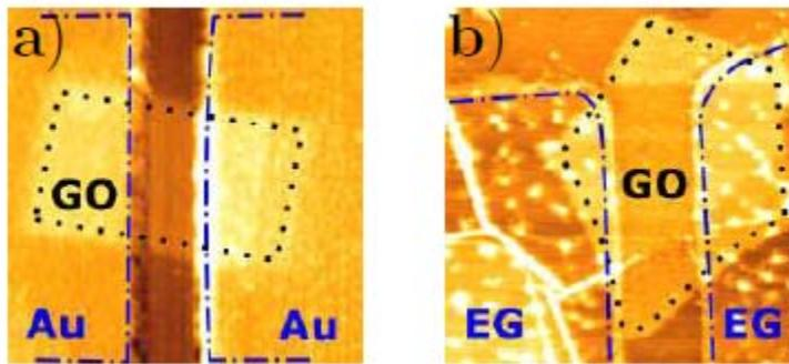
**Fig4: a) a bilayer rectangular GO flake (outlined by a black dotted line) over a 400nm Au gap. Blue dash dot lines represent Au pads. b) A pentagonal GO flake bridges 2 EG electrodes<sup>11</sup>.**
