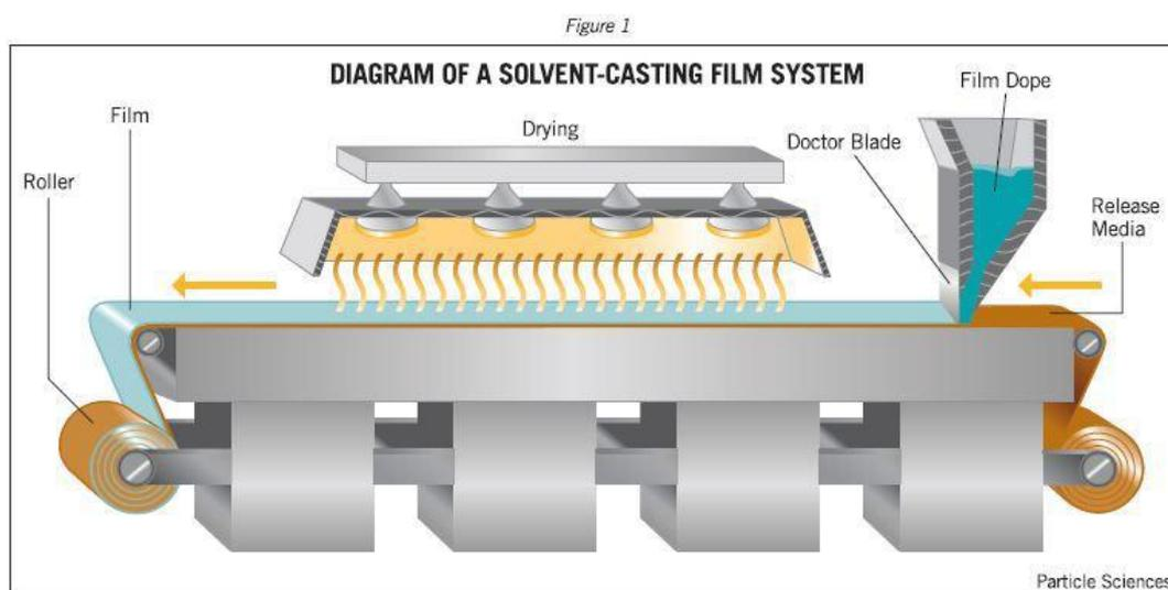
Figure 4: Solvent casting method (Bhusnure et al., 2017)
