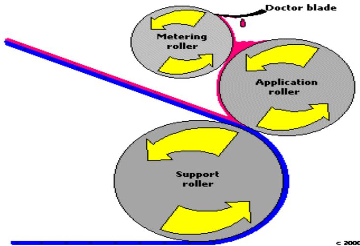
Figure 6: Three roller coating films forming the unit (Bhusnure et al., 2017)
