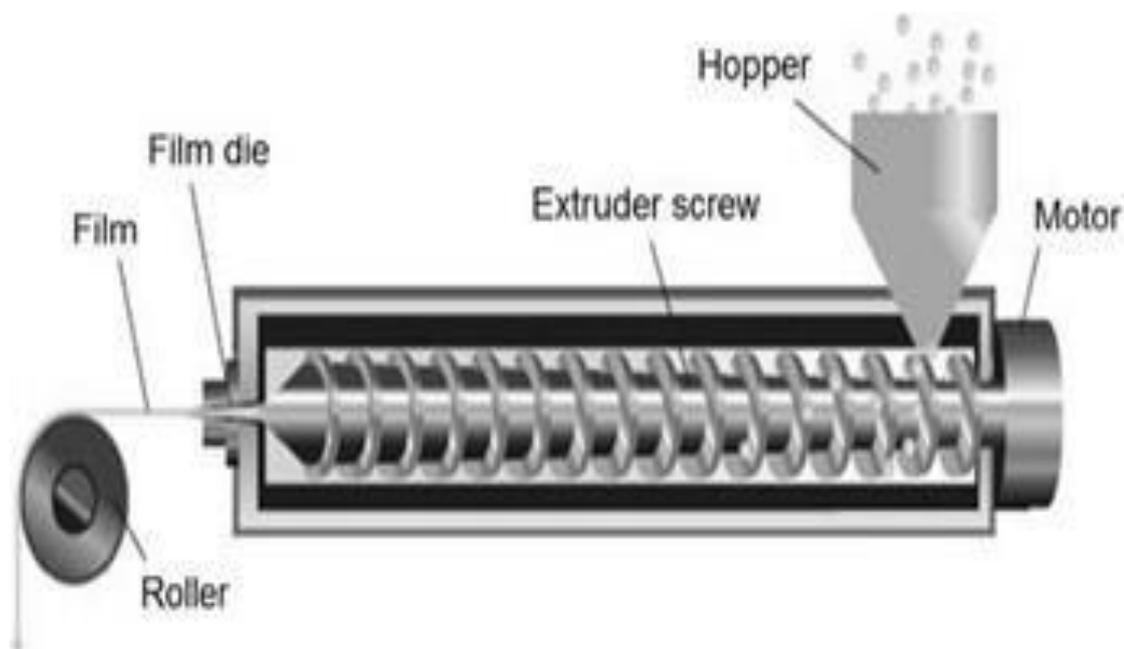
Figure 5: Hot melt extraction machine (Thakur & Tyagi, 2019)
