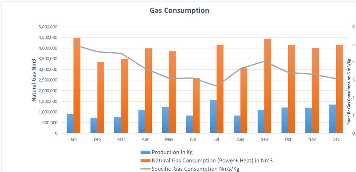
Figure 4.4. Plot of the Specific Gas Consumption of the factory from Gas Consumption (Heat +Power) right axis and Production in kg left axis during the months of 2018.
