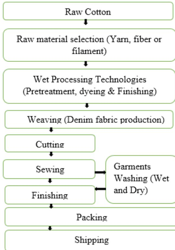
Figure 2.1. Process Diagram of Composite Textile Factory
