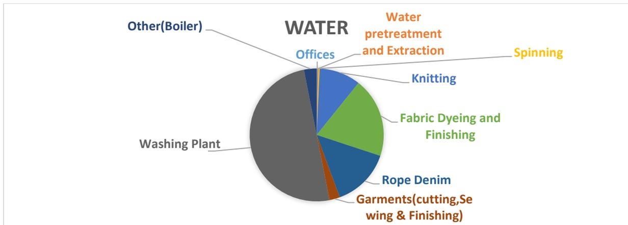
Figure 2.6. Pie chart of water consumption in percentage of utilities of the factory.
