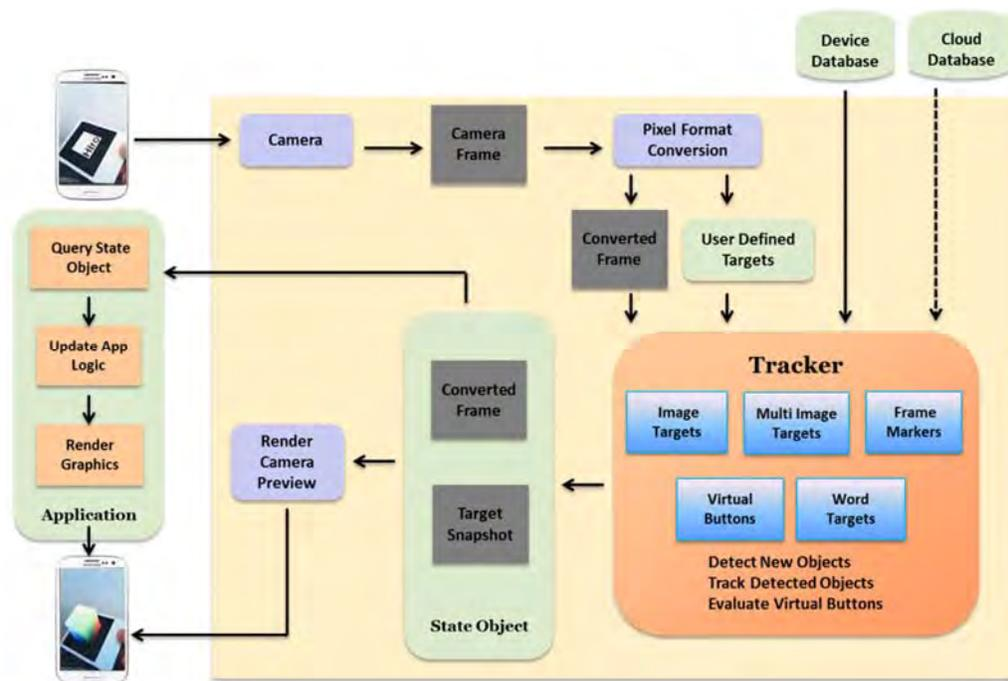
Figure 2.3 Flowchart for Target Detection
