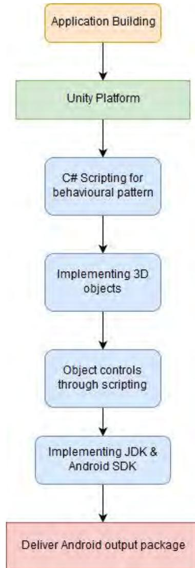
Figure 2.5 Workflow of final app development and packaging using Unity
