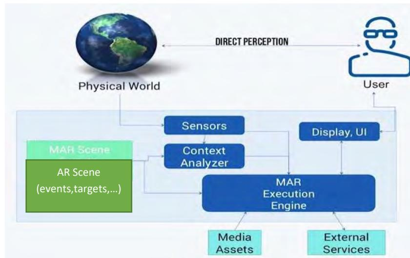
Figure 1.3 Mixed and Augmented Reality Reference Model
