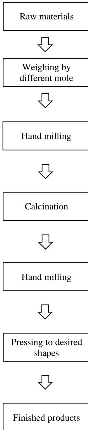
Figure 1: Flowchart of the stages in preparation of spinel ferrite
