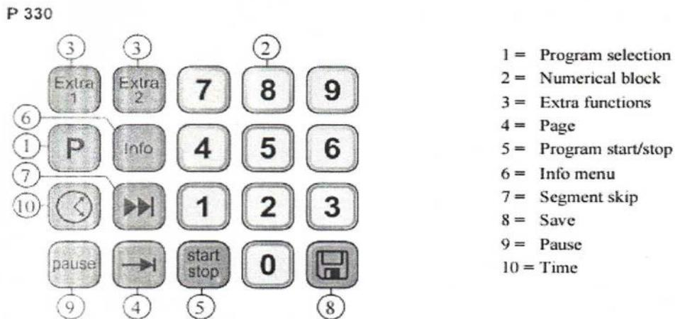
Figure 7: P330 Keyboard Block
